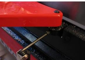
FIGURE 21: REMOVING GUARD FOR RABBETING
