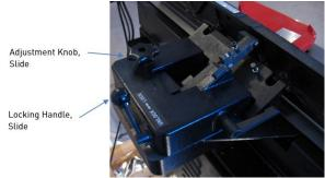
FIGURE 15: FENCE SLIDE COMPONENTS
